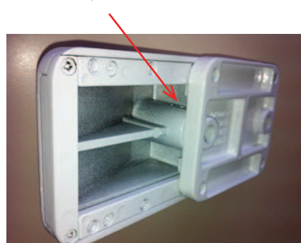
Position of push button on Thule Door Lock
